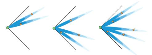
Figure 4 - Examples of MU-MIMO patterns
